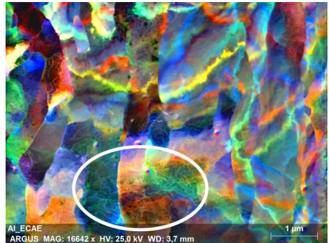
Figure 5. FSE image in transmission mode showing a network of dislocation walls (highlighted).
