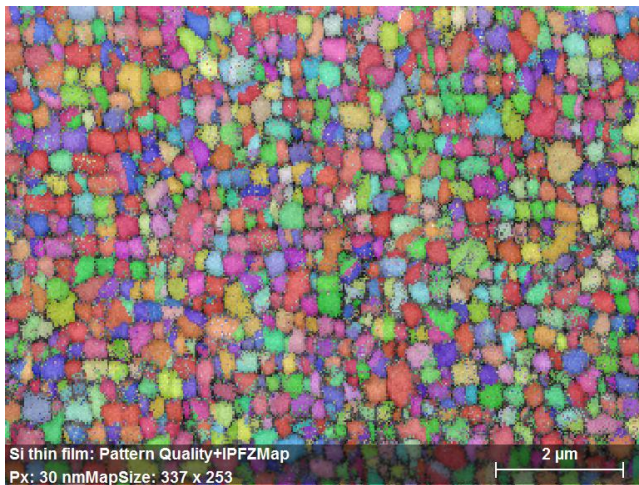
Figure 3. Standard EBSD orientation map of the Si film.
